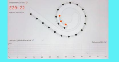
• Upon the 4<sup>th</sup> attempt with the same electrode, full insertion was achieved with correct positioning, confirmed by impedence and autoNRT
