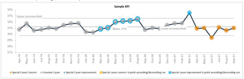
**SPC Chart** – A time series graph to effectively monitor performance over time with three reference lines; Mean, Upper Process Limit and Lower Process Limit. The variance in the data determines the process limits. The charts can be used to identify unusual patterns in the data and special cause variation is the term used when a rule is triggered and advises the user how to react to different types of variation.
