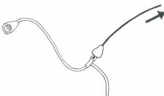
4. Screw the slim tube back onto the hearing aid.
