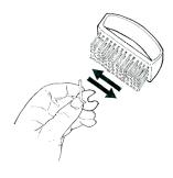
4. Connect the earmould back to the hearing aid by pushing the soft tubing back onto the hooked part of the aid.
