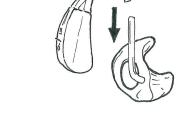
2. Wash the earmould (with the tubing still in place) in warm, soapy water -hand soap.
