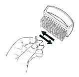
**4**. Connect the earmould back to the hearing aid by pushing the soft tubing back onto the hooked part of the aid, as shown.
